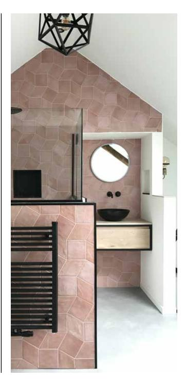
As a rule, it is recommended to start from an edge or corner. It is important to keep an eye on the sight lines. So where one enters the room, the tiles must be placed as well as possible so that this provides a nice sight line. We prefer to process the fitting pieces at edges that are not immediately visible.
